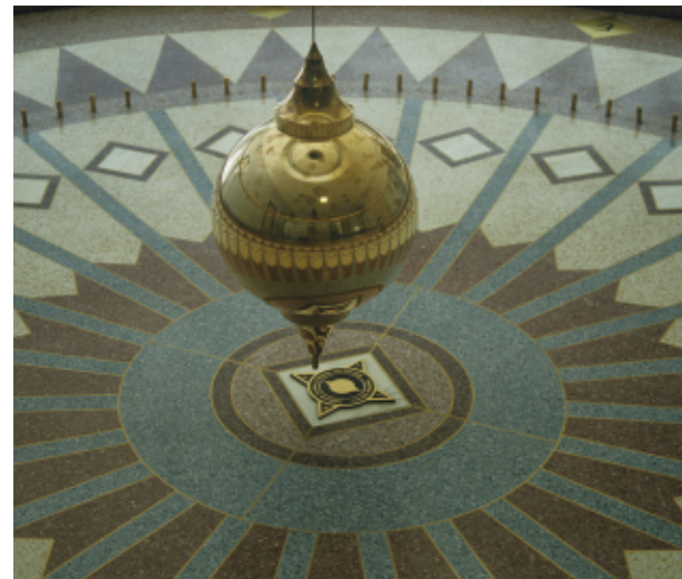
Figure 1 The 12 ft arc of this Foucault pendulum in Spokane, Washington, appears to change throughout the day. However, the actual path of the pendulum does not change. Instead, it is the floor that moves as Earth rotates under the pendulum.
