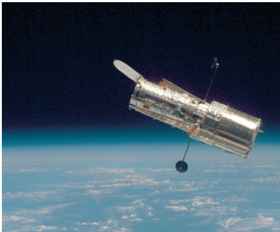
Figure 7 The Hubble Space Telescope is in orbit around Earth, where the telescope can detect visible and nonvisible electromagnetic radiation without the obstruction of Earth's atmosphere.
